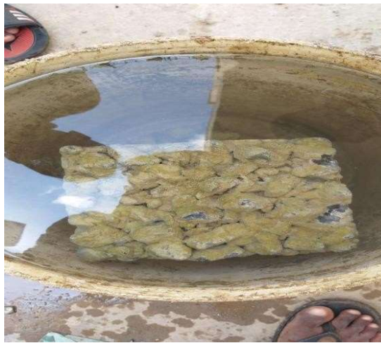
Fig. 7. Cube for Water Absorption
