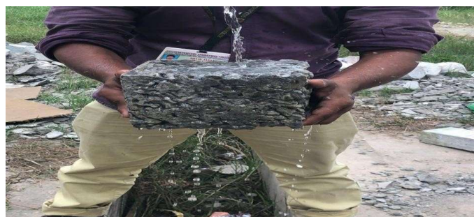
Fig. 2. Water flowing through pervious concrete cube
